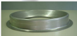
Gas turbine part from a cobalt alloy (Haynes 230). Many alloys from aluminium, steel, nickel, titanium are explosive formed
