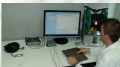
Data acquisition system with strain gages, hydrophones, geophones etc. for on-line process monitoring
