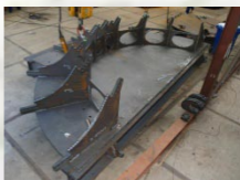
Welding jig set up for shape analysis by photogrammetry
