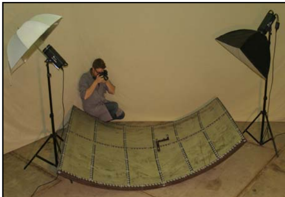
Figure 7. a VV panel in accordance with a reference ITER design of 2007; photogrammetry measurement
