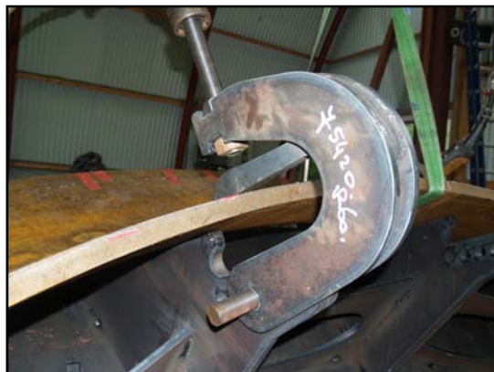
Figure 10. One of the clamps of the assembly jig
